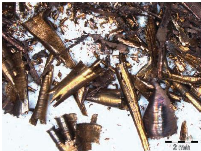
Figure 1 | Metallic machining debris.
